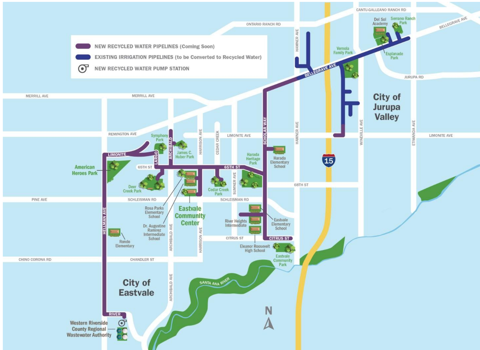
Figure 6-4: Phase 1 Recycled Water System
