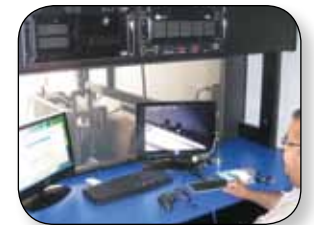
The control room of the CCTV inspection system, located inside the truck. The camera captures images inside the sewer lines.
