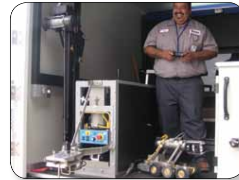
Rudy Soria, JCSD Sewer System Video Technician, testing the video camera.
